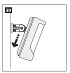
2.6. Slide the device down to fix it
