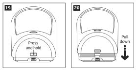
To insert the SIM card, first remove the front cover of the device (containing the detector lens)
