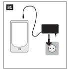
2.7. Insert the plug into the mains socket
