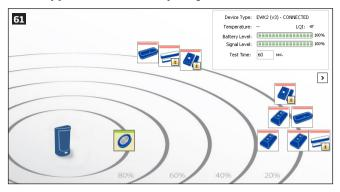
Alternatively, you can switch to radar view by clicking on the Radar View button.
