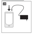
2.4. Plug the power supply connector into the device
