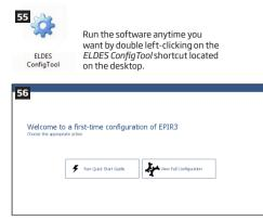
On successful first-time connection, a Welcome to first-time configuration of EPIR3 window will show up. Left-click on the Run Quick Start Guide button and follow the step-by-step instructions to program the EPIR3 system. After completing all steps, your system will be ready for use.
