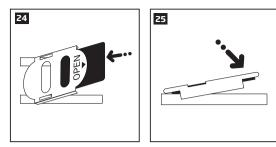
Then insert the SIM card into the holder. Insert SIM card so that gold contacts are face down when SIM card cover is flipped back down.
