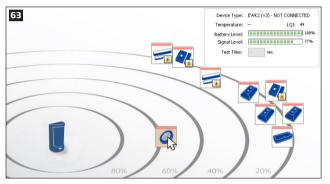
IMPORTANT FOR EWK1/EWK2: After left-clicking on the Add button it is necessary to press any button on the EWK1/EWK2 keyfob several times. After the successful wireless device binding process, the stripe above the wireless device icon will turn green. In addition, the following information related to the bound wireless device will appear:
